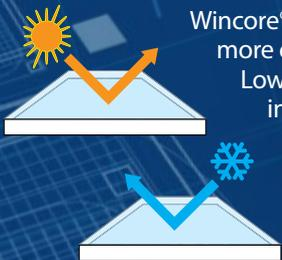
Wincore® Series 500 windows are more energy efficient with optional Low E glass and an Argon gas-filled insulating glass unit. This helps to improve efficiency by keeping homes warmer in winter months and cooler in the summer months — very important to every homeowner.
